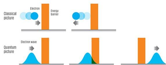
Figure 4. The effects of quantum tunneling (IEEE Spectrum, 2017)
